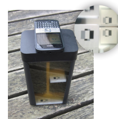
Secchi3000 and a mobile phone on the top of the device. Inside the container there is the measurement structure with plates consisting of white, grey and black target areas.
